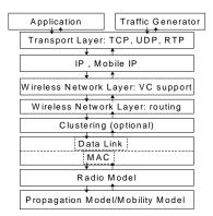
Figure 1. GloMoSim Architecture
