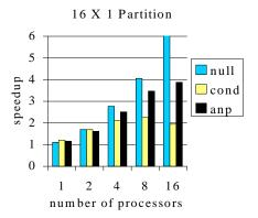
Figure 7 Speedup measurement using different partition schemes
