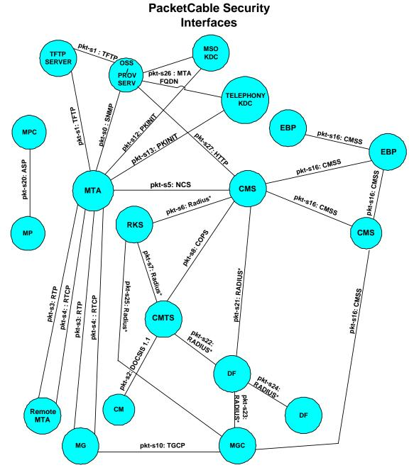
Figure 2. PacketCable Secured Interfaces
