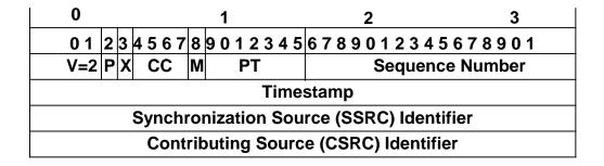
Figure 15. RTP Packet Header Format
