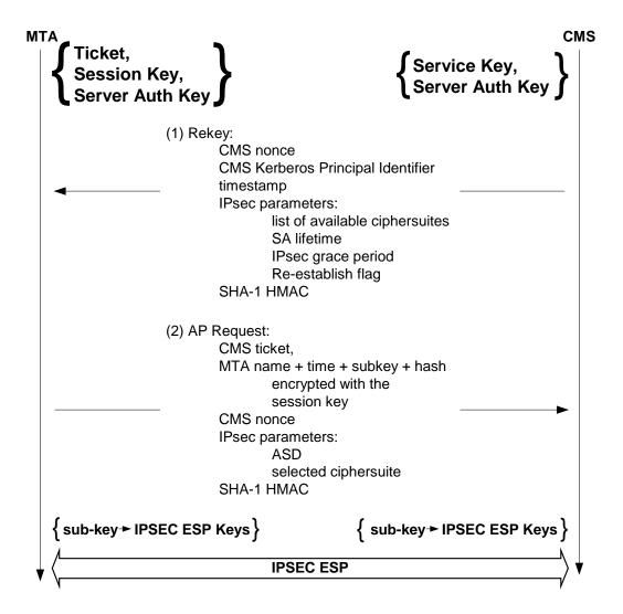
Figure 9. Rekey Message to Establish a Security Parameter
