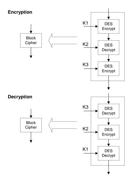
Figure 27. 3DES-EDE as Block Cipher
