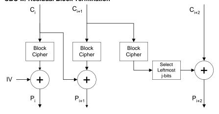
Figure 28. CBC with Residual Block Termination
