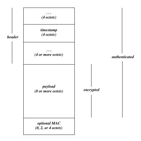
Figure 16. Format of Encoded RTP Packet
