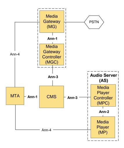
Figure 21. Audio Server Components and Interfaces
