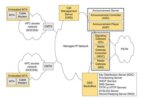
Figure 1. PacketCable Single Zone Architecture
