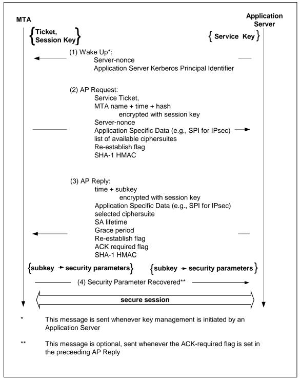
Figure 8. Kerberos AP Request / AP Reply Exchange
