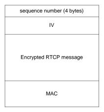
Figure 19. RTCP Encrypted Packet Format
