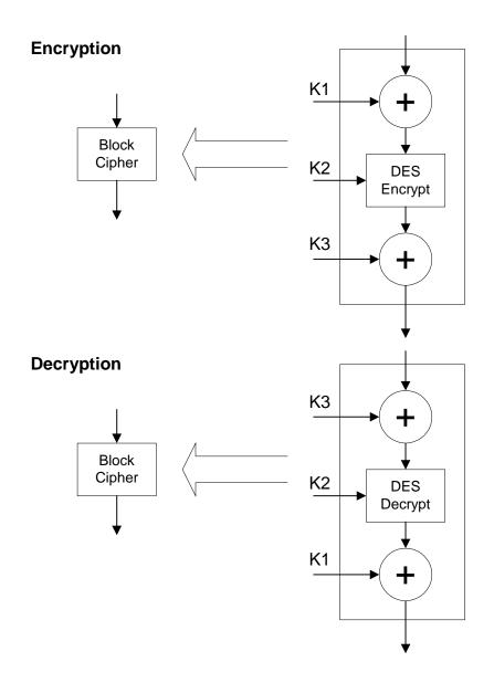
Figure 26. DESX-XEX as Block Cipher
