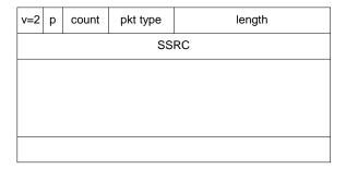
Figure 18. RTCP Packet Format
