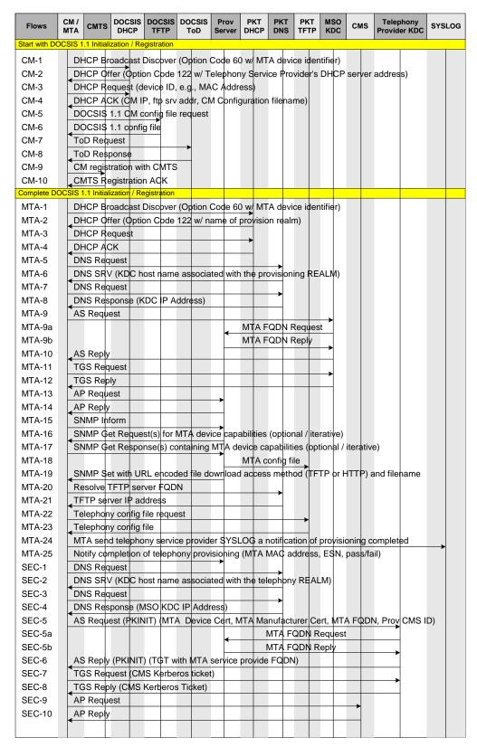
Figure 10. PacketCable Provisioning Flows
