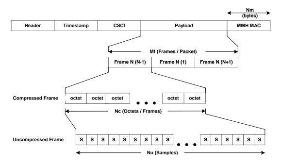
Figure 17. RTP Packet Profile Characteristics
