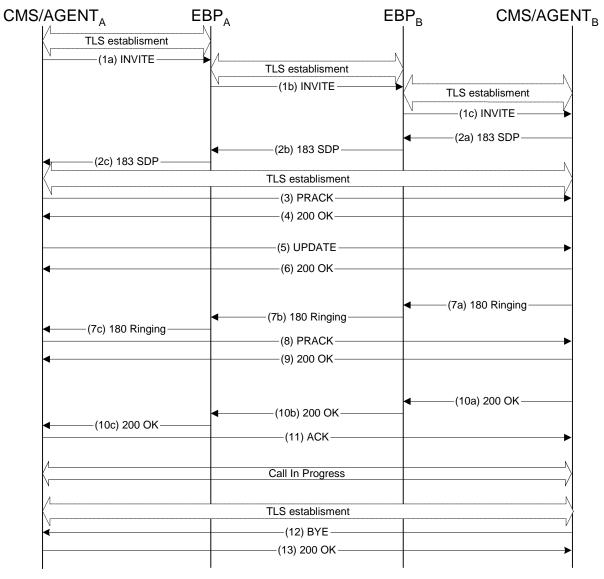
Figure 14. CMS - CMS Signaling Flow with Security
