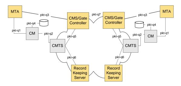
Figure 11. QoS Signaling Interfaces in PacketCable Network
