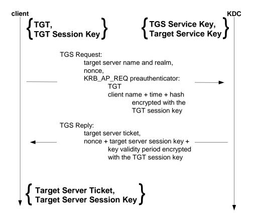
Figure 7. Kerberos TGS Request / TGS Reply Exchange
